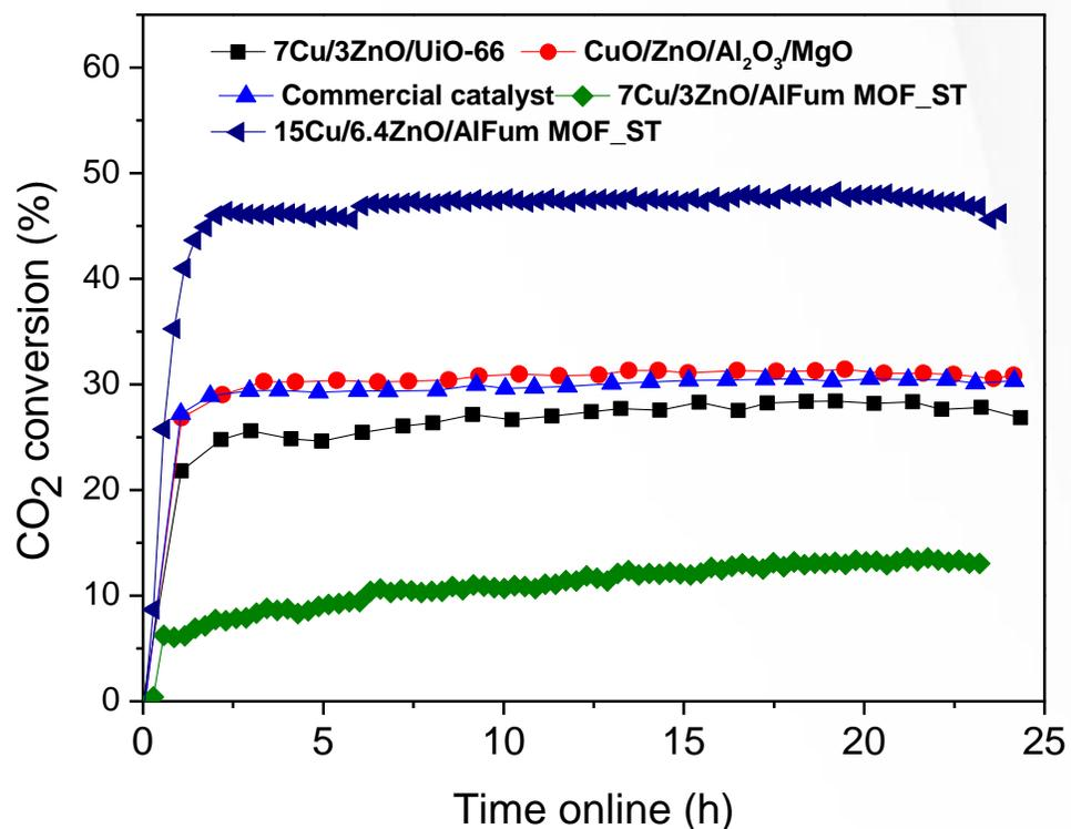
CO<sub>2</sub> conversions.  $T = 230^\circ \text{C}$ ;  $P = 50 \text{ bar}$ ;  $Q_{v,0} = 40 \text{ ml.min}^{-1}$ ;
