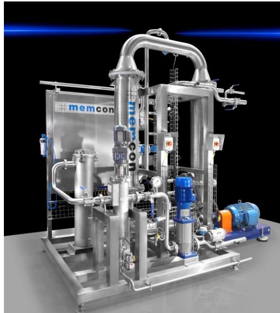
Typical ceramic UF membrane plant for treating 25 t/day spent caustic
