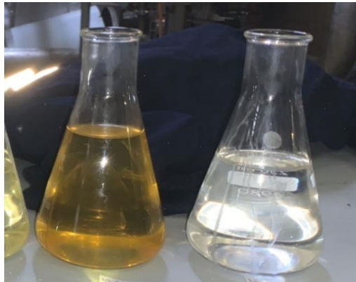
Rinse water after chem. cleaning
