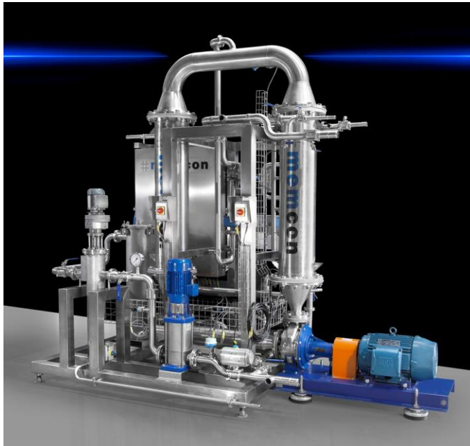
Typical ceramic UF membrane plant for treating 25 t/day spent caustic
